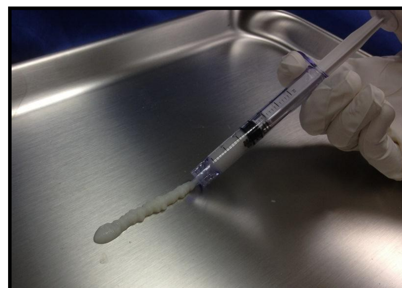
Figure 2: Gel Prototype application following reconstitution (7% w/v, 100mM NaOH)
